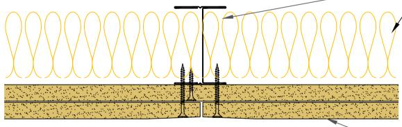
2x12.5mm Knauf Wallboard fixed with SPEEDLINE Drywall Screws at 300mm centres (200mm centres at external angles). Ref to table for fixing length.
